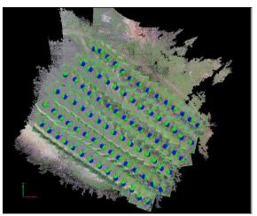
Fig. 7. Overlap in the aerial imagery. Each dot represents an image taken by the U.A.V. (87 total).
